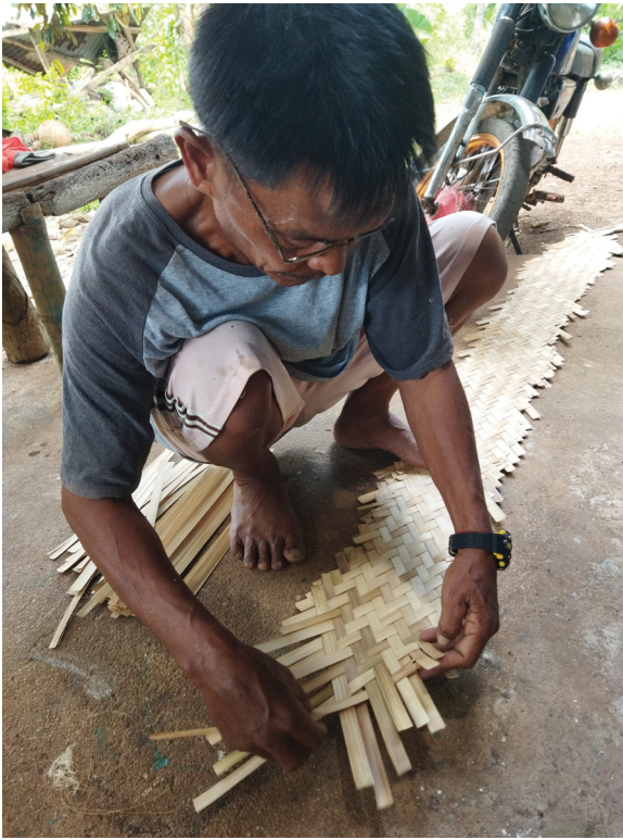
Figure 5. Working on the amakan sheets, May 2022
