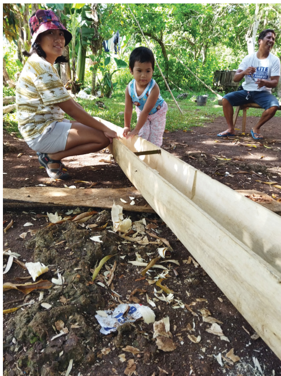
Figure 3. My wife and our daughter look into the polished hull of the bigiw , May 2022. Carving out the hull is a literal back-breaking task. The boatbuilder, at his current age, had to tip his nephew some cash to finish the carving
