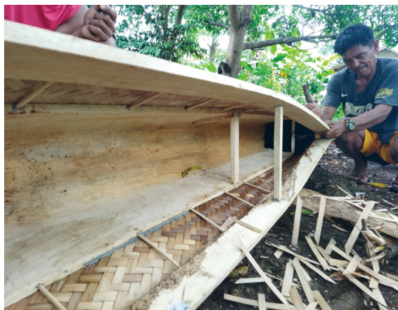
Figure 4. The interior of the bigiw shows the gusok (ribs) that serve as the frames for the amakan sheets. May 2022
