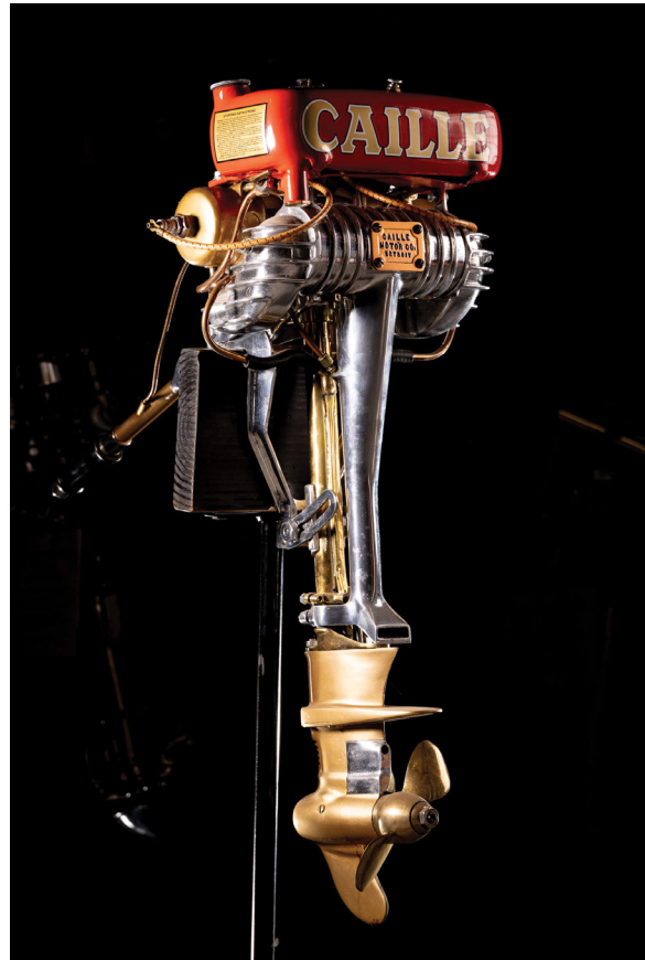
In 1910, brothers Adolph and Arthur Caille founded the Caille Perfection Motor Company. Although they had no experience in designing engines, they turned their ingenuity to producing high-quality inboard engines and, by 1913, had produced their first outboards. A noteworthy innovation on this engine is the use of a variable pitch propeller to change both the direction and the speed of the boat, at a time when reliable gear boxes were not available to engines of this size. Variable pitch is a common concept today, but was somewhat ahead of its time in 1930. Caille’s habit of painting the gas tank red led to the moniker “Redhead” for its outboard motor line. Caille Model 15 “Redhead” 5 speed, ca. 1930. Mystic Seaport Museum, 2023.57.15
