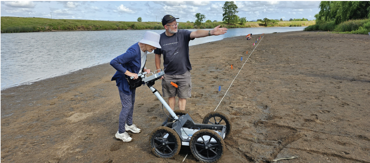
Figure 4. GPR survey of the sandbank opposite Morpeth at Taggarts Point showing Baseline 1 and pin flags that indicate the start of each survey lane. Image: Brad Duncan, 2023
