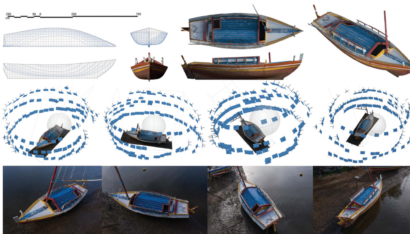
Figure 4. Process of generating the 3D models and representations. The process involves taking many 2D photographs from all angles, creating a "point cloud." Using special software, the photographs are then stitched together into a detailed 3D model. From that model, the dimensions, hull shape, and lines of the boat can be extracted. Image: Marcelo Bastos
